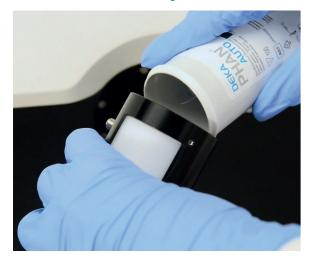
Diagnostic pads are very sensitive to air humidity, which can cause false positive results. Unlike most urinalysis machines which rely on passive humidity protection with silica gel bags, the Laura XL employs cutting edge active humidity protection technology.
